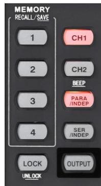
3. Press and hold an option from 1 to 4 key until the pressed option key's indicator light to store the present state of the power supply in the specified memory location.
