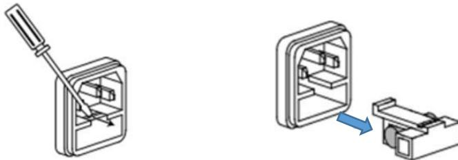
Remove and insert the proper fuse into the fuse holder.
