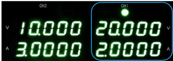
6. Press the **CH2** key (backlight lit in red), and use the current knob to set the main output current.
